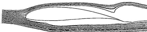
Fig. 7.26 Instantaneous streamlines over Wortmann airfoil (FX63-137)—laminar flow (unsteady results) ( Re = 100000 , M = 0.5 , \alpha = 0.0 deg.) Non-dimensional time T_n = 7.04
