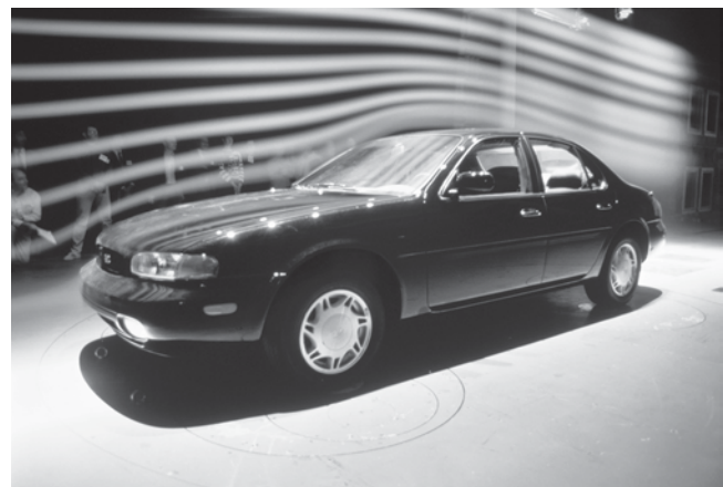
FIGURE 16-2. In a wind tunnel, the aerodynamics of a car can be evaluated by examining the streamlines of the air flow, here made visible by the addition of smoke to the air.
