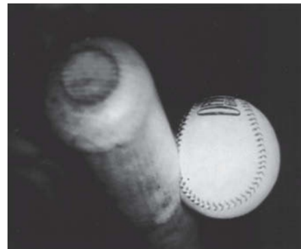
FIGURE 6-1. A high-speed photograph of a bat striking a baseball. Note the deformation of the ball, indicating the large impulsive force exerted by the bat.
