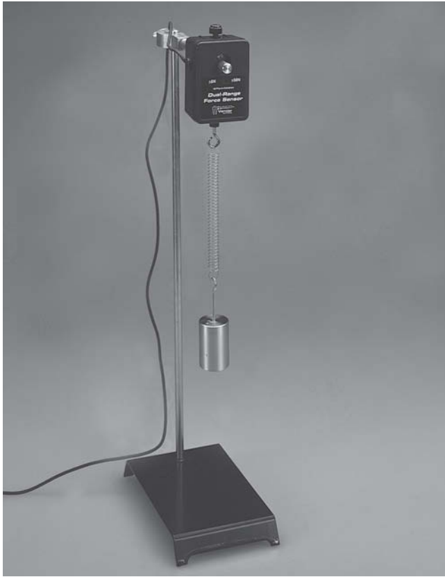
FIGURE 3-5. A mass hangs from a spring attached to an electronic probe, which can be interfaced to a computer for measuring forces. Courtesy Vernier Software and Technology.
