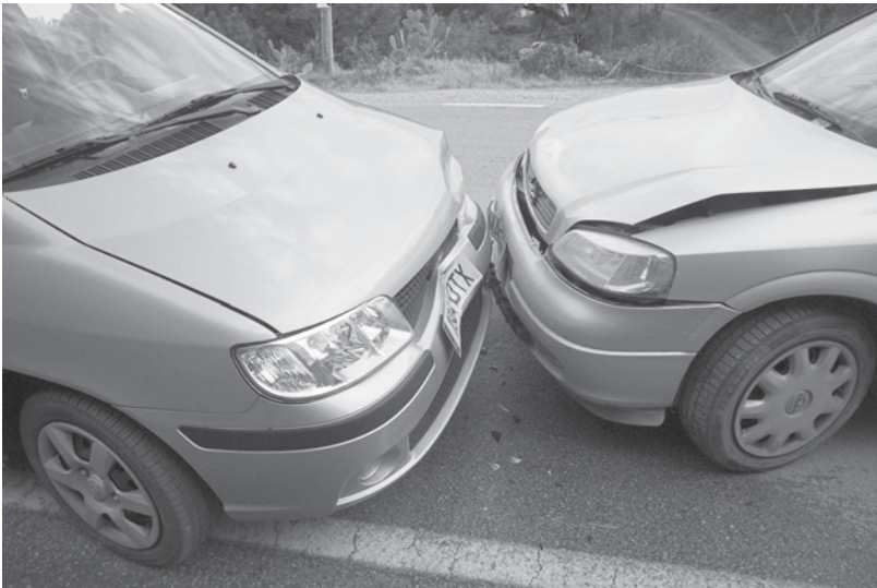
FIGURE 6-5. A collision between two automobiles. Momentum conservation is used by accident reconstruction experts to calculate the velocities before the collision.
