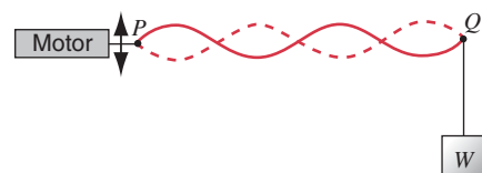
FIGURE 18-23. Sample Problem 18-4. A string under tension is connected to a vibrator. For a fixed vibrator frequency, standing wave patterns will occur for certain discrete values of the tension in the string.
