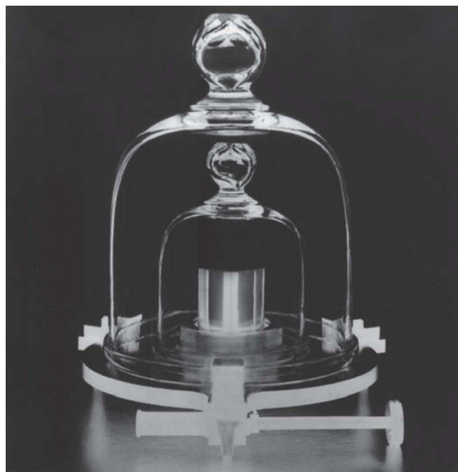
FIGURE 1-4. The National Standard Prototype Kilogram No. 20, resting in its double bell jar at the U.S. National Institute of Standards and Technology.
