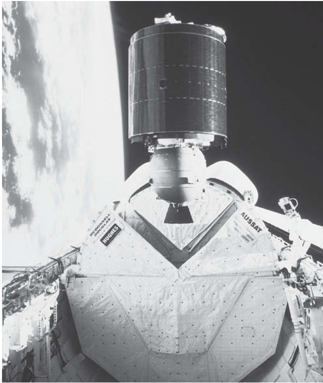
FIGURE 10-15. Deployment of a communications satellite from the bay of the space shuttle. The satellite is made to spin about its central axis (the vertical axis in this photo) to stabilize its orientation in space as it makes its way upward to its geosynchronous orbit.
